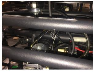
11. Route the fuel vent line down and install on 90° termination fitting.
