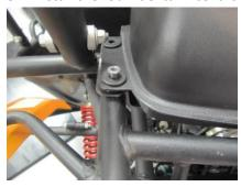
6. Install a washer onto each of the four bolts, and insert bolts through tank and frame.
