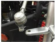
13. Install Tie Rod End/Ball Head through hole. Add flat washer, locking washer, and Castle Nut
