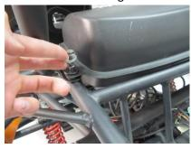
7. Loosely install the four R-washers and nuts from the bottom side of the frame.
