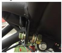
3. Torque the bolts to the required specification
