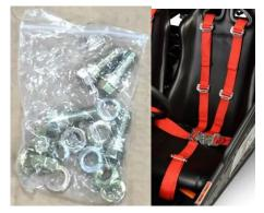
2. Feed the seatbelt through the seat and fasten to mounting hole as shown.
