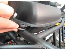
5. Install the four fuel tank collars as shown below.
