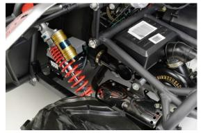
4. Tighten mounting bolts to specified Torque
