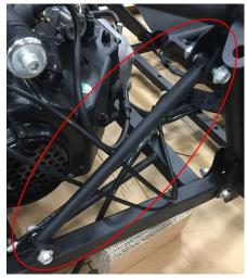
3. Mount the Rear Left and Rear Right Shock Assemblies.
