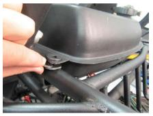
5. Install the four fuel tank collars as shown below.
