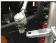
9. Install Tie Rod End/Ball Head through hole. Add flat washer, locking washer, and Castle Nut
