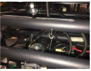
11. Route the fuel vent line down and install on  $90^{\circ}$  termination fitting.
