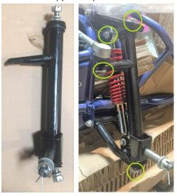
5. Tighten Nut to Torque Specification
